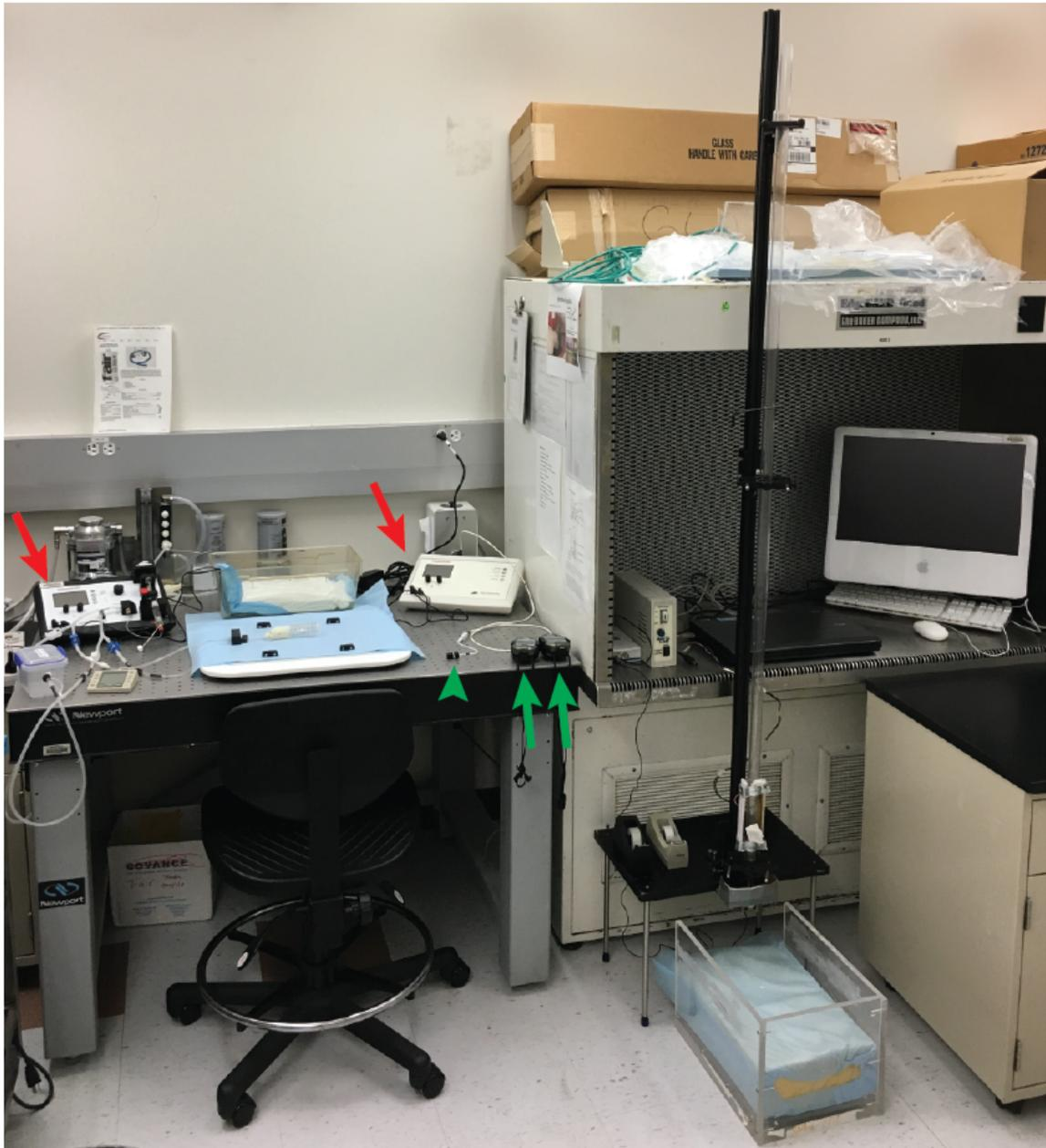
**Figure 3.2. Injury system, anesthesia and physiological measurement systems.** The complete injury setup includes the weight-drop injury apparatus and two computers used
