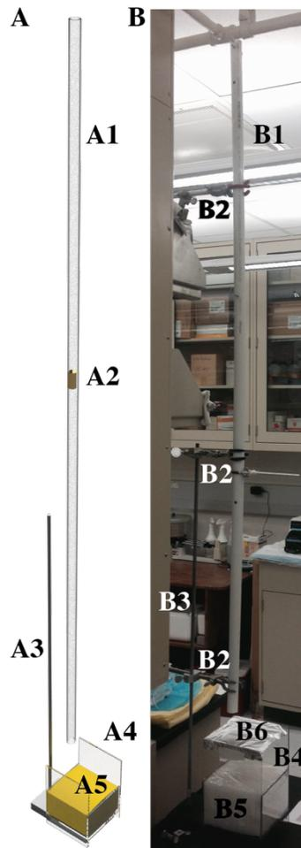
**Figure 2.1. Initial TBI apparatus.** A) A 3D render of the first apparatus before its construction. B) The apparatus after assembly and in place in the lab. A1-B1) polyvinyl
