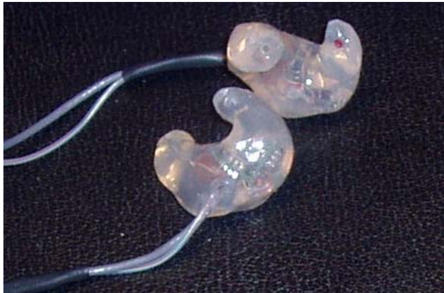
Figure 4: Custom molded earpieces with embedded sensors
