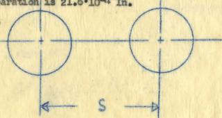
Constant separation of flares at 30 feet and 3 frames before MK II burnout.
