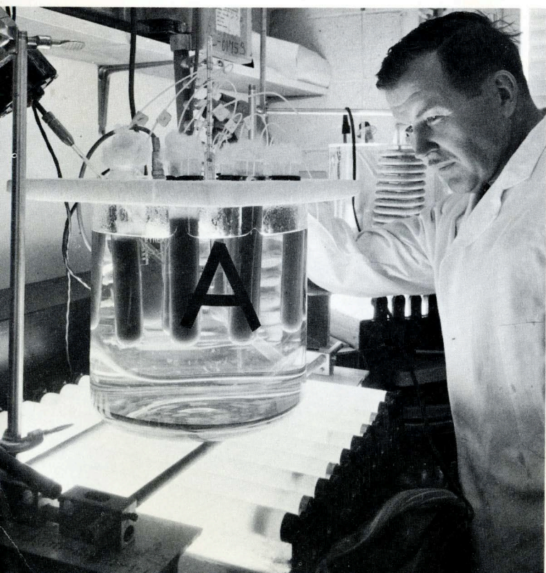
This photo shows the photosynthetic gas exchange system at Martin's Space Medicine Section in Denver. The test tubes contain algae, growth of which is promoted by light from fluorescent tubes. Checking the system is Dan Richardson, chief of bio-engineering.
