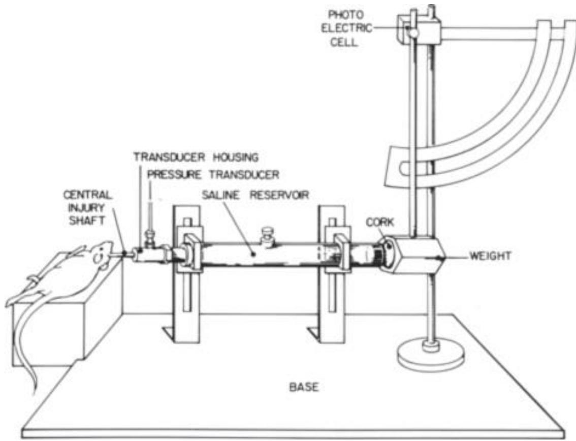
Figure 1 - Shows a diagram of the fluid percussion device that was used in these experiments (Dixon 1987).
