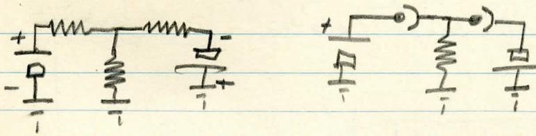
Tried Barb. Col. 'Micro positioner', a polarized relay coil D.C. res of  $\approx 200 \Omega$  would operate readily on .4 W which is current sens. of  $\frac{.4}{200} = .002 A = 2ma -$
