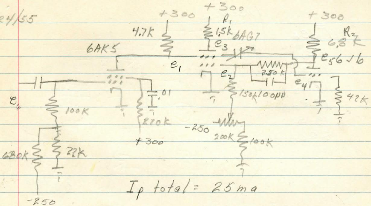
Tried this ckt - Output Amplitude was insufficient even with larger values of  $R_1$  -  $e_5$  sloped badly
