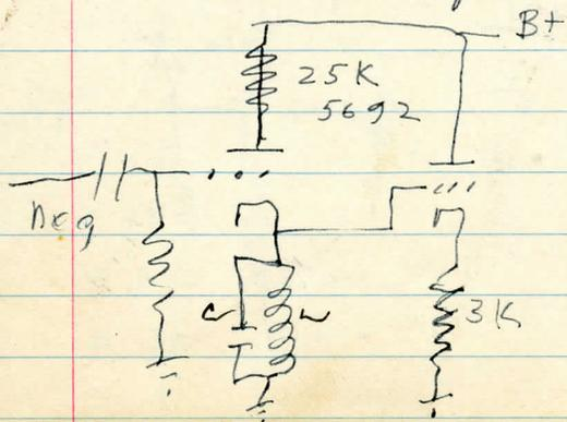
By using ckt below with various values of  $C$  &  $L$  sine waves with ~~various~~ almost negligible ~~values~~ damping -
