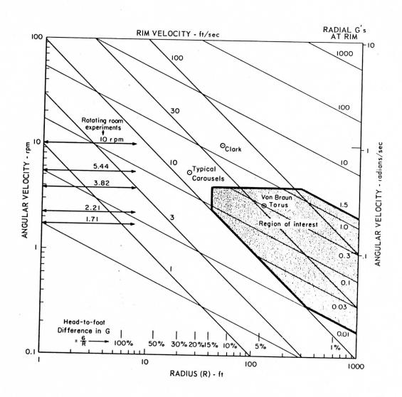
In the figure are presented results of a study which estimated general limits for the various parameters describing a rotating space station on interplanetary probe.
