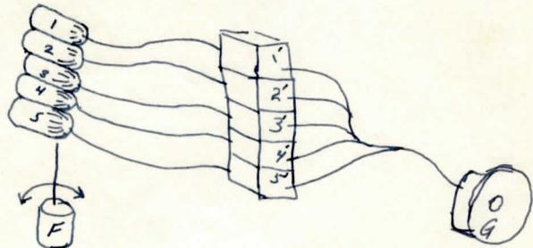
A-E represents an area scanned by the photo cells 1-5, A being the area scanned by 1, B by 2, etc. These cells are driven by a scanning device F. Electrical output of the cells control the amplitude of five oscillators, <sup>each</sup> of different frequency. Their electrical outputs are in turn combined and fed to the earpiece G.
