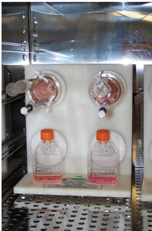
Figure 2.1: Photographic depiction of experimental set-up in the incubator. One flask served as the control flask, one flask was irradiated, one bioreactor represented modeled microgravity alone, and the other bioreactor was irradiated.
