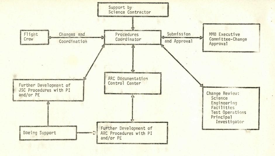
Figure 2. Flow Chart for Final Development and Change Control of Inflight Procedures
