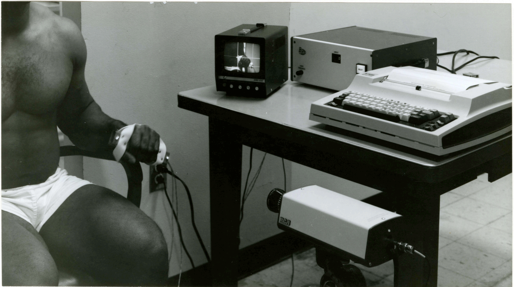
Fig. 1. Photograph of the Automatic Video Goniometer in use. The subject is holding a bar with reference lamps which are being scanned by the TV camera and displayed on the monitor with the angle of the lights being measured and printed by the microprocessor control and terminal shown.
