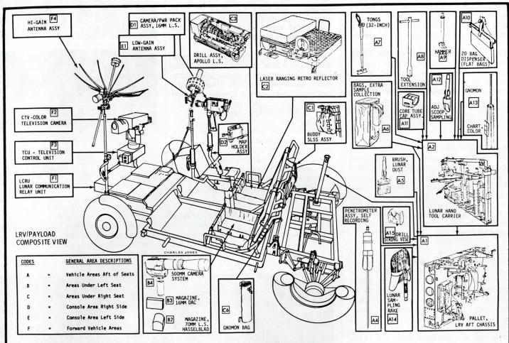
A variety of scientific instruments and other equipment is carried on the lunar rover by the astronauts of Apollo 15.
