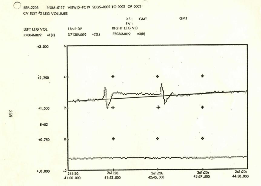
Figure 3.5.1-1a. - Same as Figure 3.5.1-1 Except A Mean Volume Line Has Been Added To Show Slow Drift And Overshoot.
