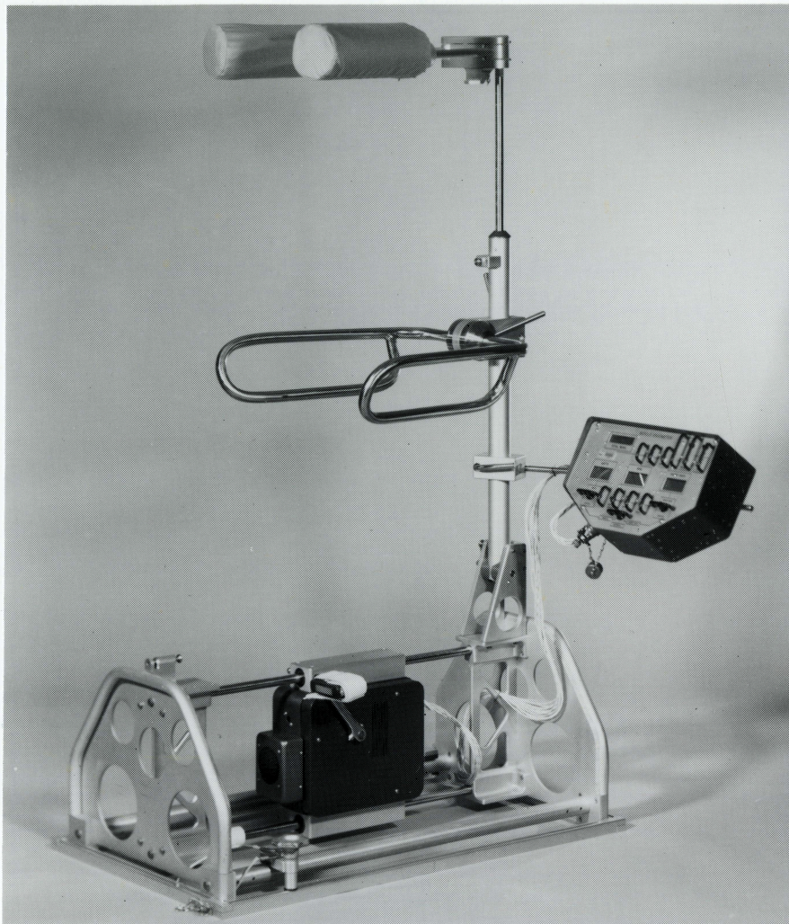
Figure 5.— SLS-1 bicycle ergometer showing the extensive restraint system.
